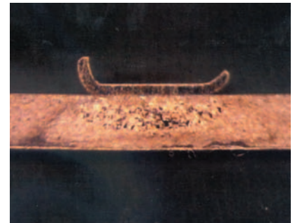
Heat affected zone closer to the weld interface with improved button size and strength.
