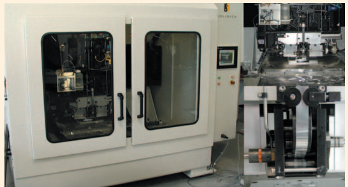
Developed with assistance from EWI, Solidica's Form-ation rapid prototyping machine can produce articles of almost any shape and size.
