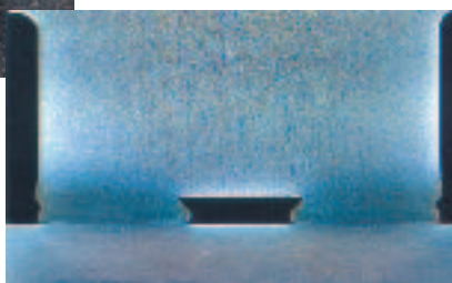
Macrosection of a Mild Steel Annular Resistance Projection Weld
