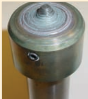
Figure 3: PCBN pin tool after 60-in. long weld
