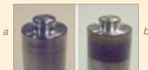
Figure 2: W-25%Re pin tool: (a) Prior to weld; (b) after 10-in. long weld
