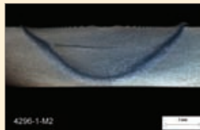
Figure 4: Macrograph of L80 friction stir weld made using CPW tool
