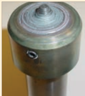
Figure 3: PCBN pin tool after 60-in. long weld
