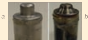
Figure 1: CPW pin tool: (a) Prior to weld; (b) after 10-in. long weld
